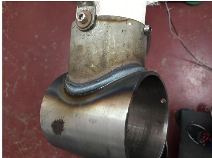
Figure 21. Pipe-connect-pipe arc welding result.
