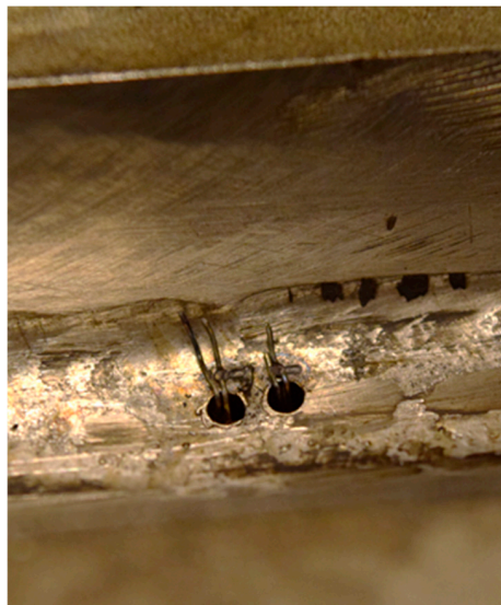
Figure 3. Example of two inserted thermocouples to register temperatures in Weld Pass 2. Holes of 2 mm in diameter were used to insert the thermocouples from the backside by drilling through the root pass. After the insertion, the thermocouples were spot welded on the surface of the joint—in this case, the surface of the root pass.
