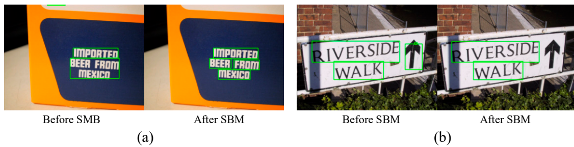
Figure 7. Examples of CRF processing effects. (a) Two lines of text are placed in one bounding box. After CRF processing, each word has a separate bounding box. (b) The arrow is erroneously detected as text and the arrow bounding box is removed after CRF processing.
