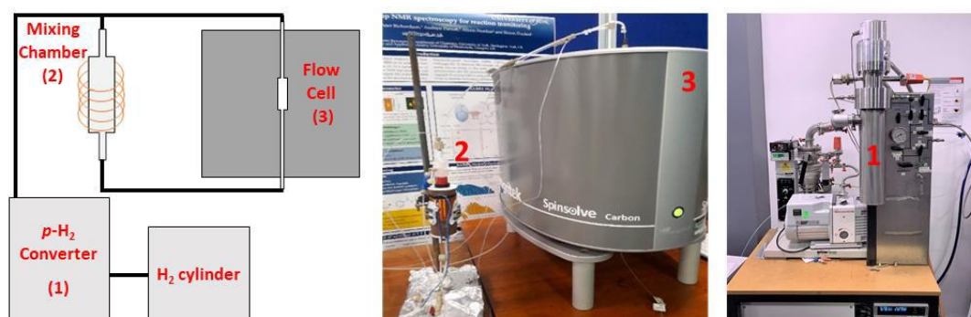
Figure S1. Schematic representation and photo of the automated flow system setup used for SABRE hyperpolarisation with detection on the benchtop NMR spectrometer.
