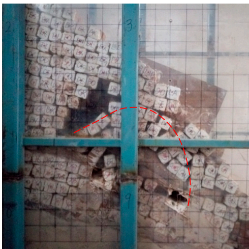
(a) Deformation after mining ore body #3
