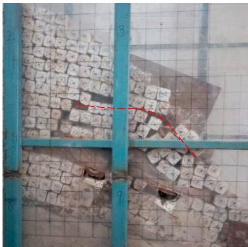
(a) Deformation after mining ore body #2
