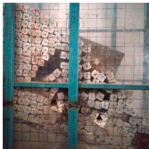
(a) Deformation after mining ore body #4
