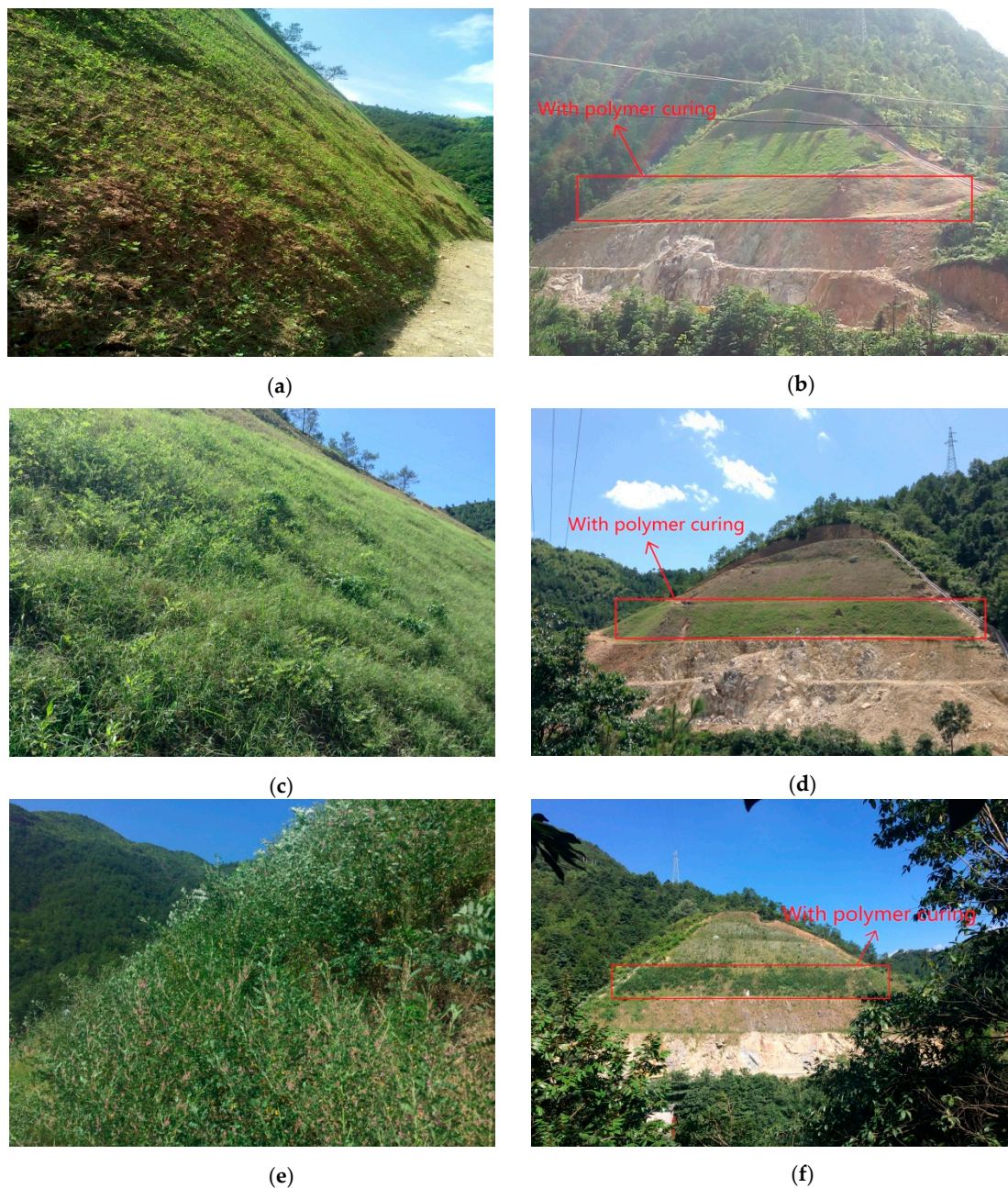
Figure 15. Plant growth conditions of the Zhejiang test slope: (a–b) 1 month later; (c–d) 3 months later; (e–f) 1 year and 3 months later.
