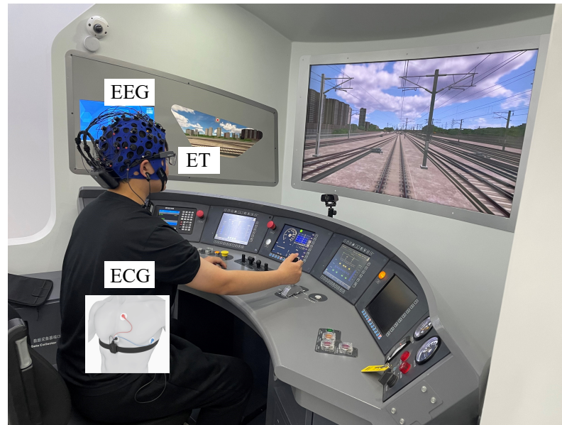
Figure 1. Experimental environment for signals acquisition under a simulated driving environment.
