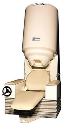
Figure 3. UCSF Magneto encephalography device using SQUIDS technology.
