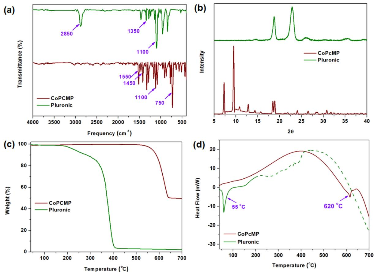
**Figure S1.** Characterization of the facilitated carrier (CoPCMP) and compatibilizer (Pluronic) by (a) FTIR; (b) powder XRD; (c) TGA and (d) DTA analysis (for the case of Pluronic, due to its onset of degradation occurs at around 200 °C; thus the DTA curve beyond 200 °C is indicated as dotted line).
