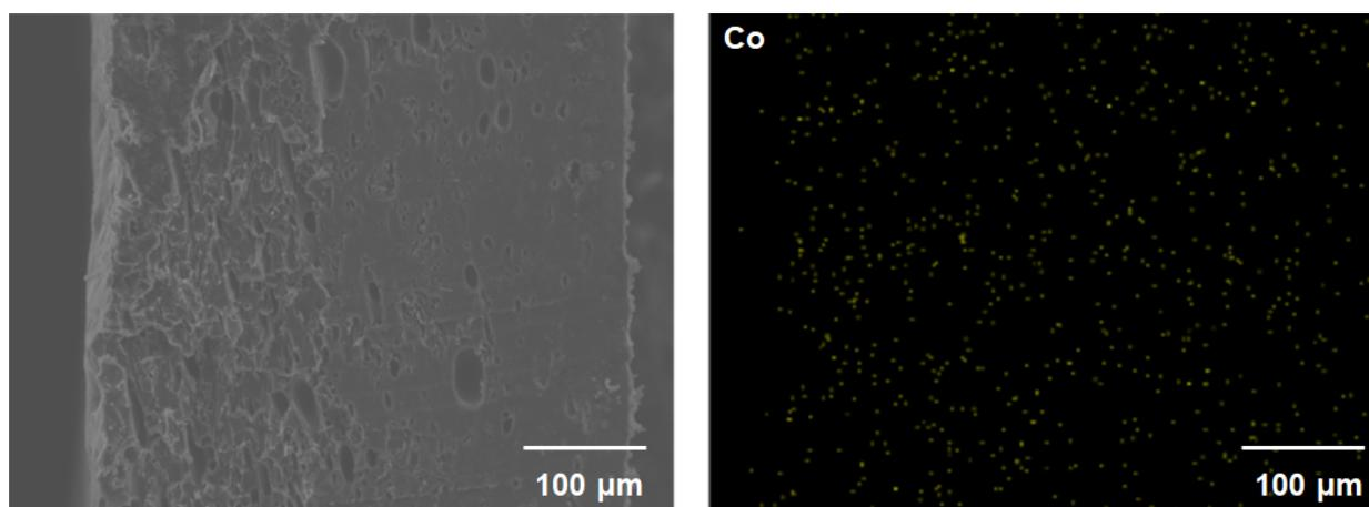
**Figure S6.** EDX mapping of 5 wt% CoPCMP and 10 wt% Pluronic in Matrimid membranes.
