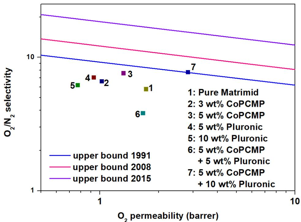
**Figure S5.** Comparison of the membrane performance (in Table 1) with the upper bound limit (1991, 2008, 2015) [1-3].
