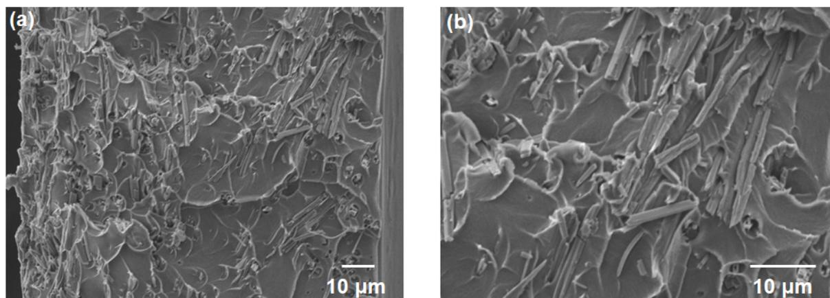
**Figure S4.** Cross-sectional FESEM image of Matrimid-CoPCMP (10 wt%) under (a) low magnification; (b) high magnification.
