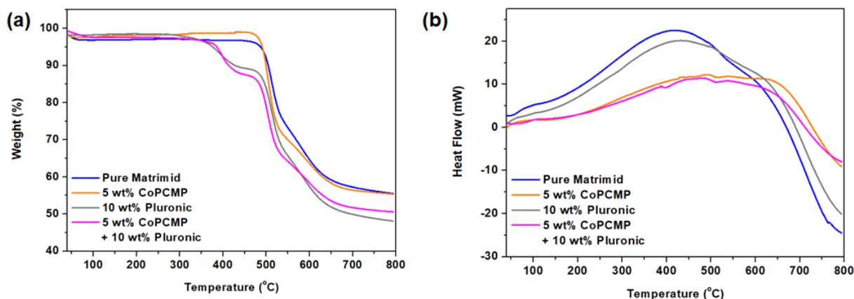
**Figure S3.** (a) TGA and (b) TDA of neat (Matrimid), blended (Matrimid-Pluronic) and composite (Matrimid-CoPCMP and Matrimid-Pluronic-CoPCMP) membranes.
