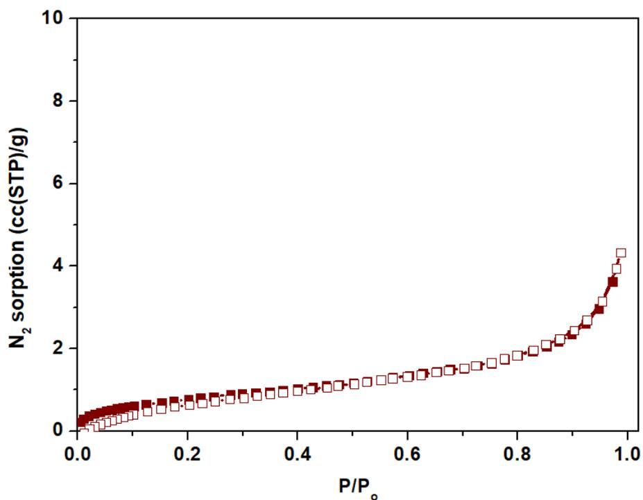
**Figure S2.** N<sub>2</sub> sorption for CoPCMP at 77 K.
