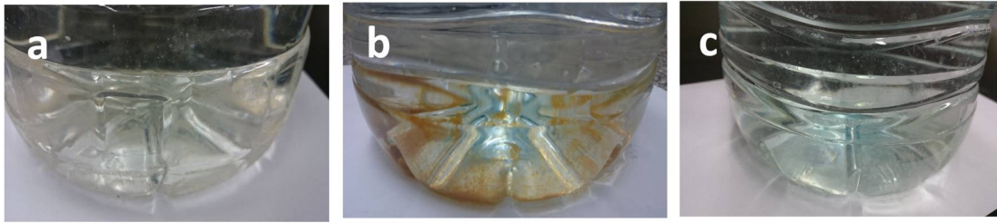
Figure S2. Photos of seawater (a) before coagulant addition, (b) after sedimentation, and (c) after pretreatment.
