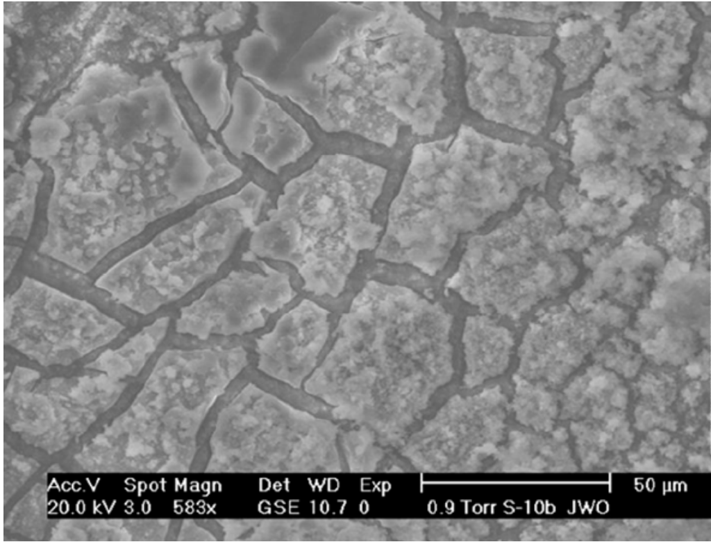
ESEM analysis of last element (dried surface with scaling).
