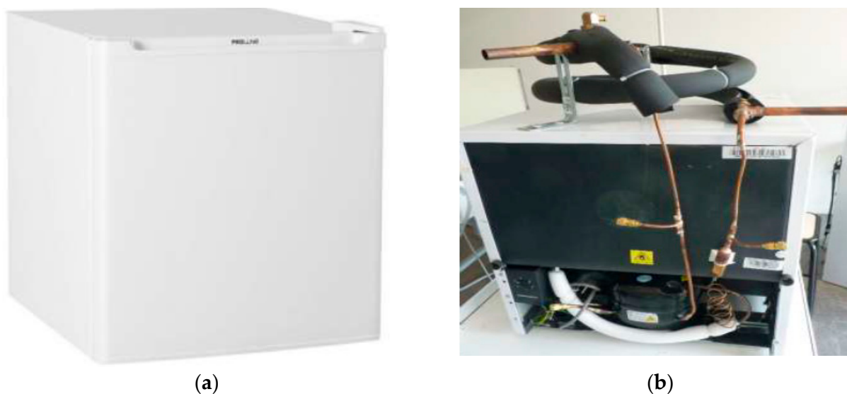
Figure 1. Heat pump for the simultaneous production of cold and heat (a) picture of the refrigerator and (b) photo of the refrigeration machine modified.
