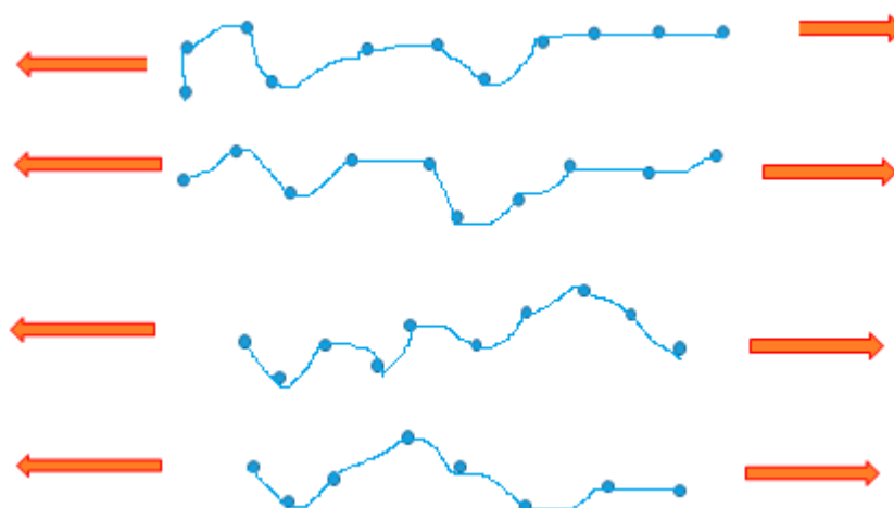
Figure 6. Rotation of the Kuhn segments resulting in alteration of polymer shape as a result of thermal vibration of atoms.
