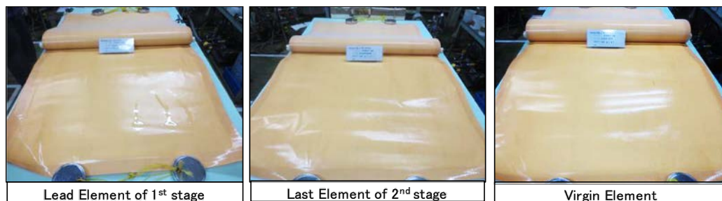
Figure 11. Surface conditions of the lead and last RO element (collection on 81st day of operation).
