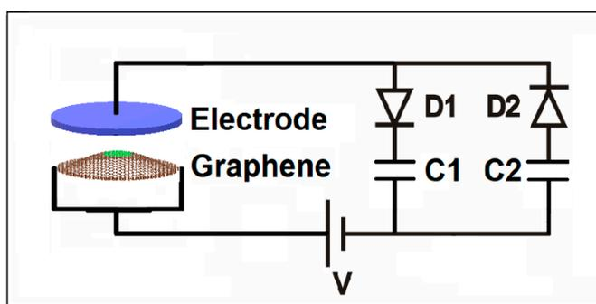
**Figure 1.** Graphene energy harvesting circuit using two diodes (D1 and D2), two storage capacitors (C1 and C2), and a rechargeable battery ( $V$ ) to charge the graphene-electrode variable capacitor on the left.
