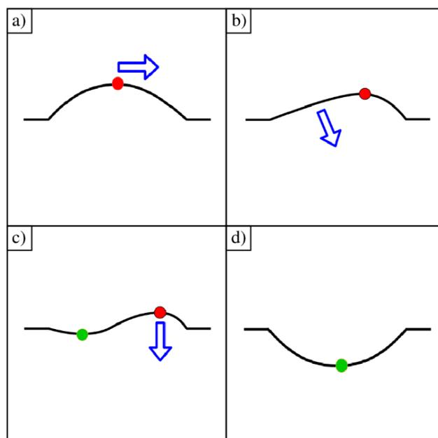
**Figure 8.** Conceptual illustration of the shape transformation through curvature inversion: (a) The maximum of the ripple moves from center to right; (b) Curvature is low on the left side. Local atoms are pulled down toward the fixed frame; (c) The left side passes through the  $x$ - $y$  plane and the ripple forms a sine-like shape; (d) The left sub-ripple has pulled the right sub-ripple down. A single ripple is formed below the  $x$ - $y$  plane.
