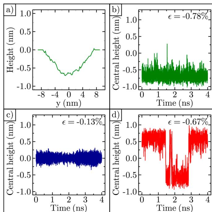
**Figure 3.** Role of strain on ripple dynamics at 3000 Kelvin: (a) Typical cosine-like cross-sectional profile of a ripple; (b) Central height of a highly compressed ripple in time; (c) Central height of a lightly compressed ripple in time; (d) Central height of a bistable ripple in time.
