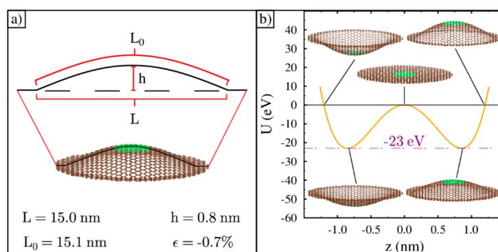
**Figure 2.** Ripple construction and the double-well potential: (a) An example graphene ripple constructed after compressing a flat sheet by 0.7% and adding a third dimension so that the arc length equals its original uncompressed length; (b) The double-well potential for the ripple. Five ripple illustrations show the shape at different points along the energy curve. The function precisely fits the five energy data points found at zero Kelvin by stretching and compressing the lattice by 0.7%.
