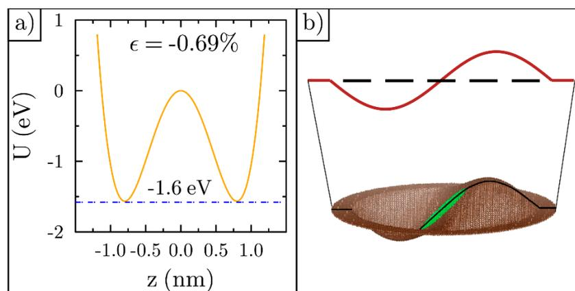
**Figure 5.** Potential energy and ripple shape: (a) Double-well potential for strain of  $-0.7\%$ ; (b) Illustration of a possible ripple shape during inversion, along with its cross-section.
