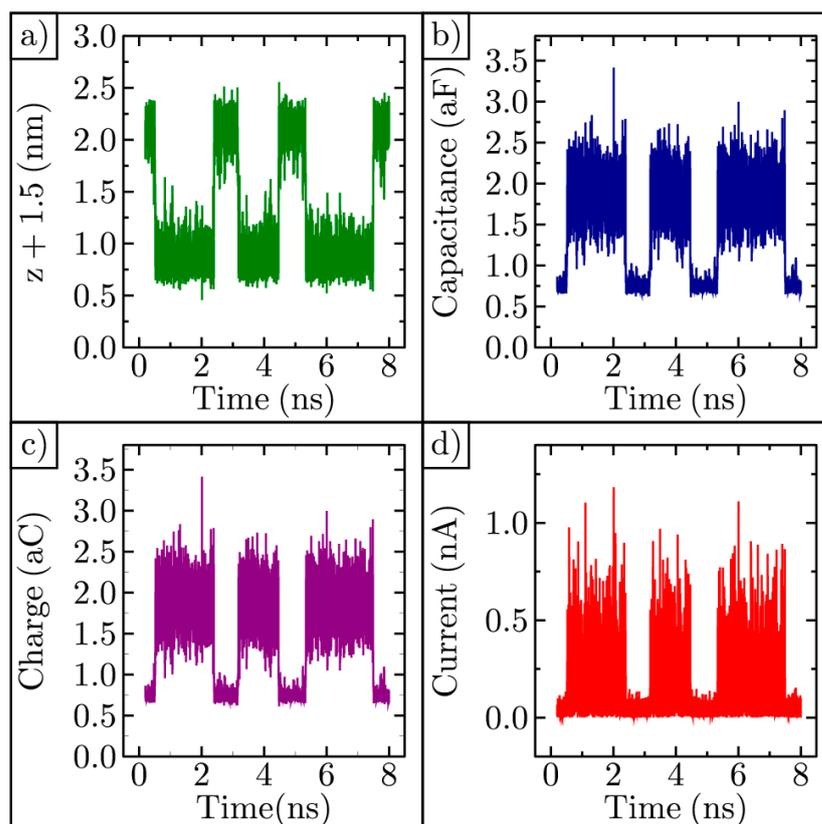
**Figure 9.** Graphene ripple near a fixed electrode: (a) The distance between the electrode and the ripple; (b) Capacitance of the graphene-electrode capacitor; (c) Charge on the graphene capacitor; (d) Rectified portion of the alternating current flowing in the circuit.
