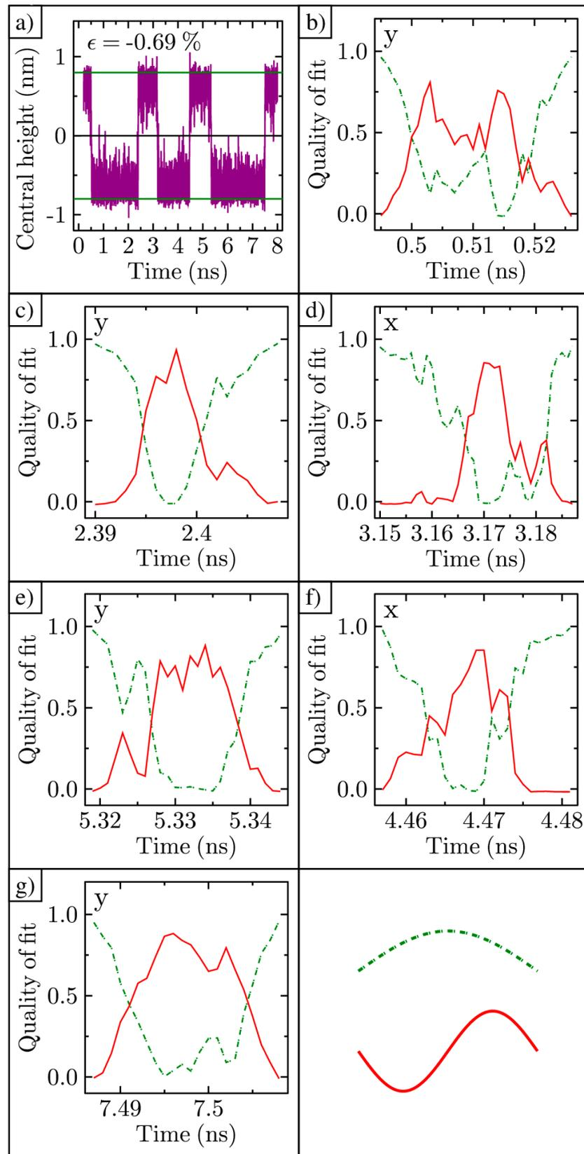
**Figure 7.** Cosine–sine–cosine shape transformation: (a) Central height of ripple in time; (b–g) Cosine and sine goodness-of-fit R<sup>2</sup> values for the x- or y-direction (as labeled) cross-section of the ripple in time. Lower right box shows the legend.
