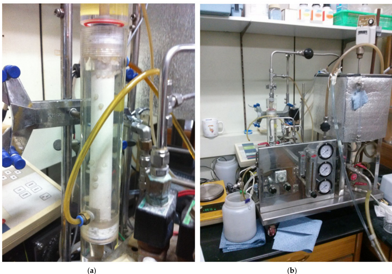
Figure 2. Combined water treatment process of tubular or seven channel MF membrane and PP beads with periodic water backwashing: (a) seven channel MF membrane; (b) total combined system.
