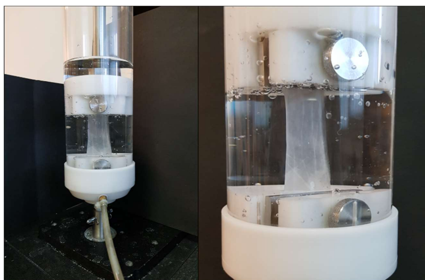
Supplementary Figure S8. Hydrogel PVA membrane mechanical assessment.
