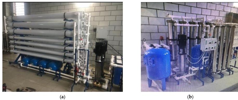
**Figure 2.** Reverse osmosis membrane units producing 4 cubic meters per hour (a) and 20 cubic meters per hour (b) of quality water with brine concentration membrane devices to reduce concentrate flow rate to 1% of the feed water flow rate or less.
