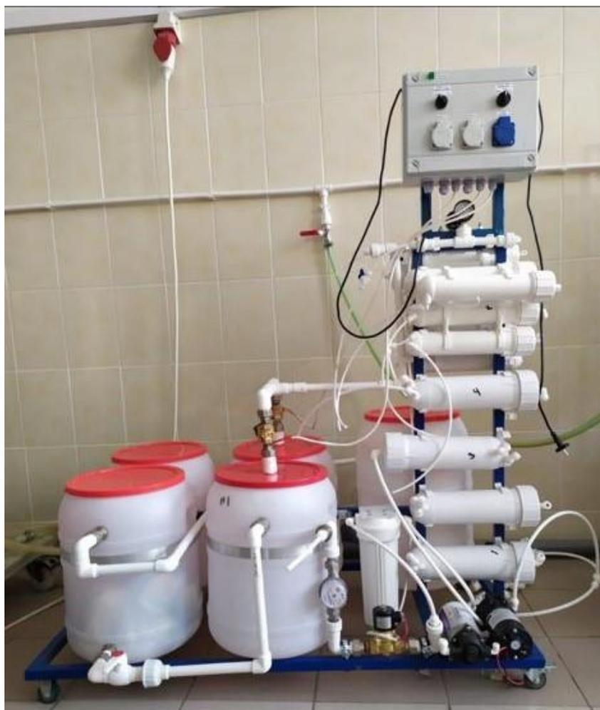
**Figure 1.** A three-stage pilot membrane unit for brine concentration using deposition of calcium carbonate in the seed reactor in continuous mode.
