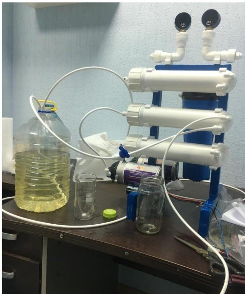
**Figure 6.** Membrane test unit with different membrane types to investigate separation of the brine into monovalent ion concentrated solution and divalent ion concentrated solution.
