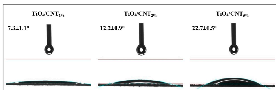
Figure 1. Contact angles formed between the given titanium dioxide/carbon nanotube (TiO 2 /CNT) nanocomposite-coated membrane surface and the ultrapure water droplet (10 μL), measured immediately (within 1 s) after dropping.
