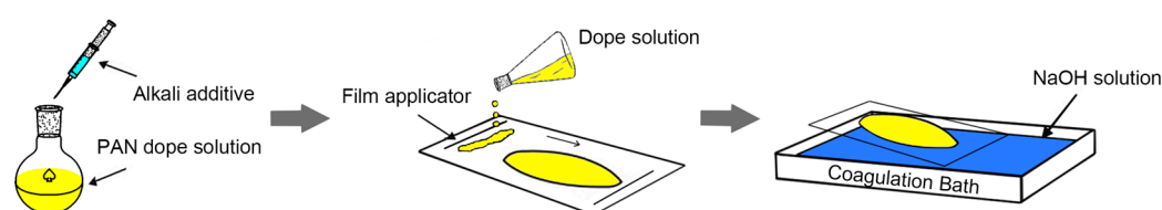
Figure 2. Procedures for preparing the pre-hydrolyzed PAN-based membrane.
