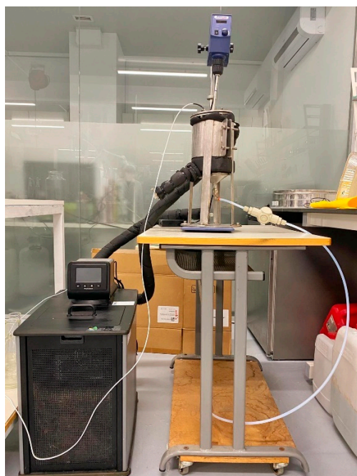
Figure S3. The real picture of apparatus used of progressive freeze concentration.
