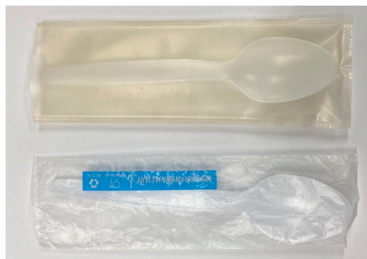
Figure 9. Transparent protective envelope made from G25CA15 film (top) compared with that made from HDPE film (bottom).
