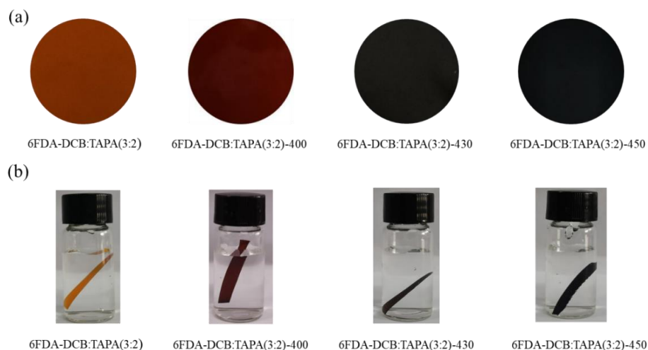
Figure 1. Optical pictures (a) and solubility tests (b) of 6FDA-DCB: TAPA (3:2) and its thermally treated membranes at 400 °C, 430 °C, and 450 °C for 2 h.
