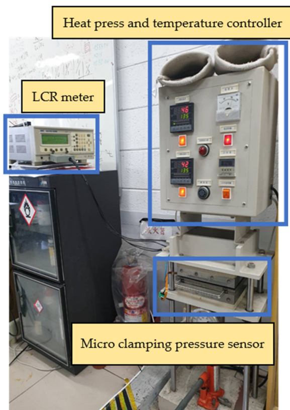
Figure 18. Experimental configuration of micro clamping pressure sensor correction.
