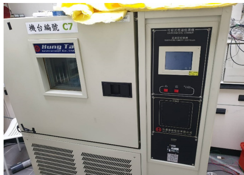
Figure 11. Program-controlled constant temperature and humidity testing machine Hung ta HT-8045A Environmental Chamber.
