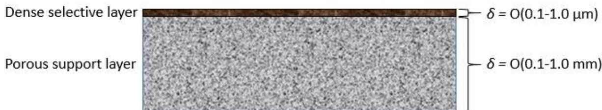
Figure 1. Representation of gas separation membrane, which typically consists of a thicker, porous support layer coated with a thin, dense selective layer.
