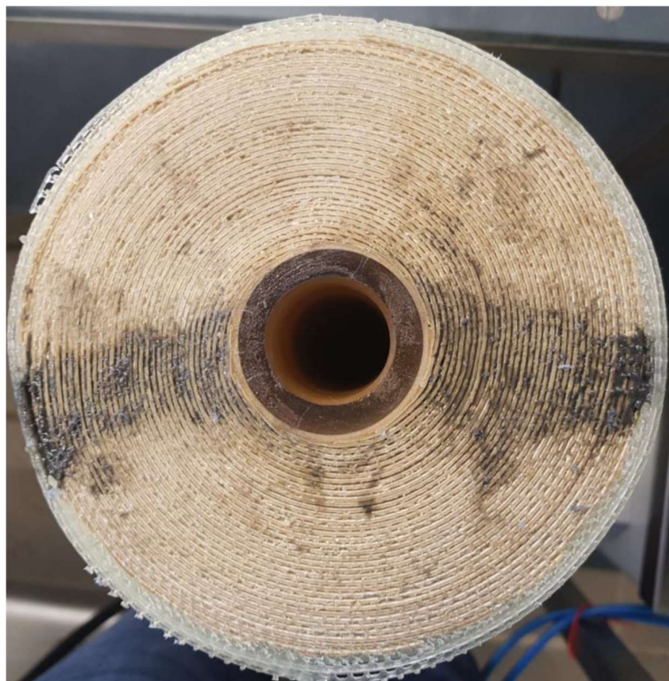
Figure 2. The membrane module was modified by adding glue dots (see black areas) radially along the membrane diameter.
