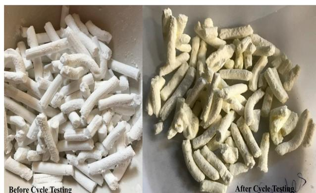
**Figure 4.** Photographs of the adsorbent pellets before and after the cyclic testing.
