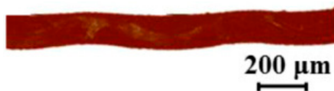
Figure 8. Cross section of swollen AMX-Sb membrane. Adapted from [20].
