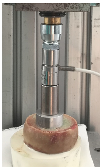
Figure 5. Femoral head (bottom) with round test implant cemented to the bone surface and the force measurement system (top).
