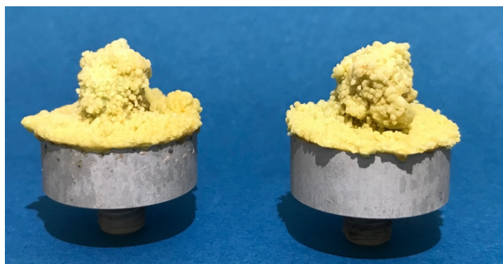
Figure 6. Already implanted test implants with cement after removal of all organic components.
