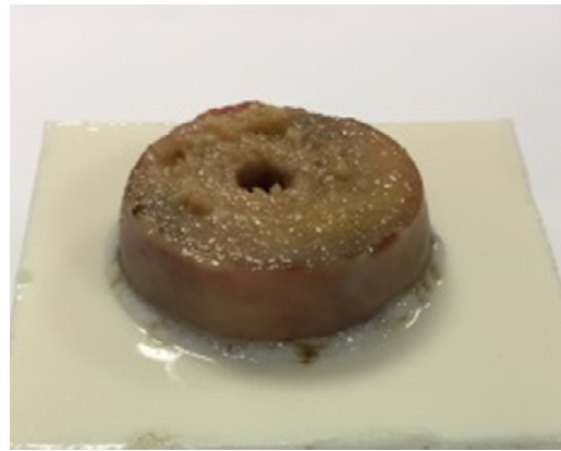
Figure 2. Embedded femoral head with drilled hole for the peg, prior to cleaning procedure.
