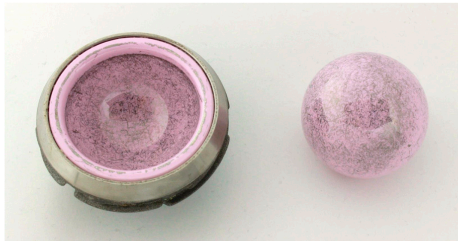
Figure 5. Ceramic-on-ceramic bearing couple with globally distributed metallic deposition on femoral head and insert.
