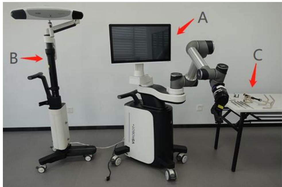
Figure 1. Robotic base station (A), optical tracking system (B), and toolset (C).
