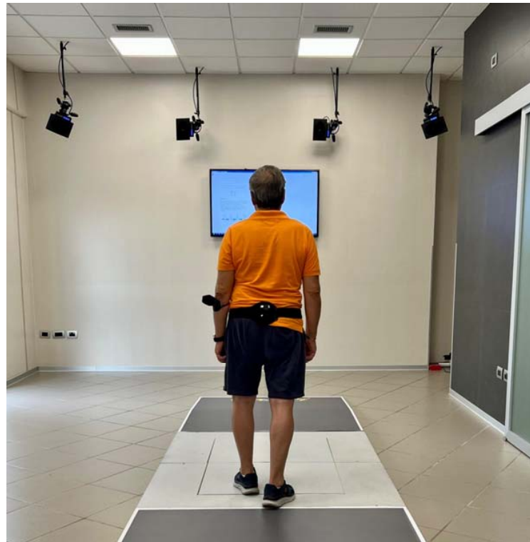
Figure 1. Gait analysis setting. The inertial measurement unit (G-Sensor, BTS bioengineering) is located on the 5th lumbar vertebra for a quantitative gait evaluation. Patients were asked to walk for 7 m. Data are elaborated with the manufacturer software (G-Studio, BTS bioengineering).
