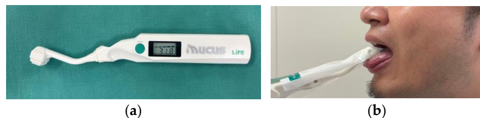
Figure 2. Measurement of oral moisture: (a) a measurement device (Mucus); (b) measurement using this device.
