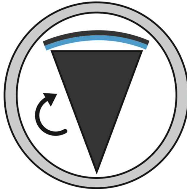
Figure 4. Schematic illustration of the single-source layered detector DECT system (Phillips Healthcare). The dual-energy datasets are achieved via spectral separation at the detector level. This system capitalizes on the polychromatic beam generated at the source and employs specialized dual-layer detectors sensitive to a specific energy spectrum. The superficial layer, which absorbs approximately 50% of the total photons, is designed to primarily absorb low-energy photons. The second layer absorbs the remaining high-energy photons.
