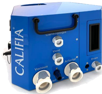
Figure S11. Calafia Patient Simulator by BioMed Simulations [11] is a mid-fidelity ECMO sim. This device can be used for both ECMO and heart-lung machine simulations. It mimics the patient's hemodynamics, physiologic response, and respiratory changes.
