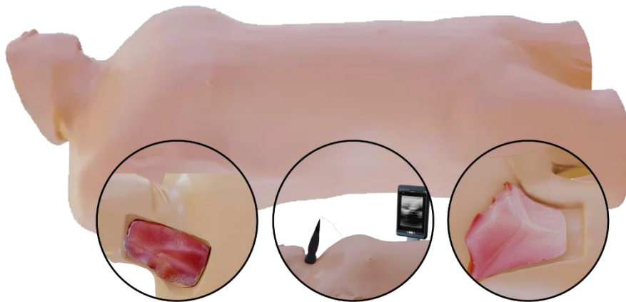
Figure S26. E-Sim Pro by The Simulator Company [26] is a mid-fidelity ECMO sim. Available options are: multiple cannulation site, connection to ECLS, heart rate control, cardiac output control, with physiological blood flow.
