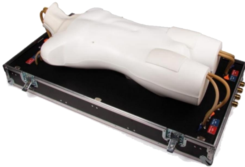
Figure S25. ECMO Trainer Professional MK2 by Erler Zimmer [25] is a mid-fidelity ECMO sim consisting of pump simulating arterial and venous circulation, an option for cannulation, and monitoring.
