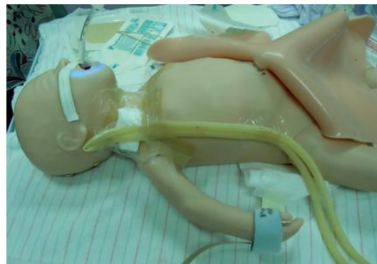
Figure S5. ECMO Initiation Simulator by Thompson et al. [5] is a low-fidelity ECMO sim, consisting of a neonatal mannikin with (partly) external cannulation sites and liquid-filled tubing mimicking the vessels for cannulation. Some parts of the tubing have been hidden by a cover (see femoral).
