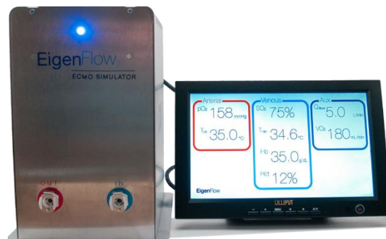
Figure S24. Eigenflow 2 ADVANCED by Curtis Life Research [24] is a mid-fidelity ECMO sim. A multifunction, wireless, and remote controlled simulator. The Eigenflow 2 ADVANCED can be connected to an ECMO circuit and has two variable controlled valved for clinical simulations. Furthermore, the 3-Dmed® ECMO cannulation kit [1] is used for cannulation training.
