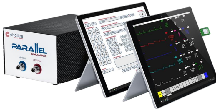
Figure S14. Parallel Simulator by Chalice [14] is a mid-fidelity ECMO sim. It is a portable and customizable simulation hub with two high-resolution tablets (control panel and monitor). The Control panel sets vital statistics and physiological parameters can be altered to simulate situations. The monitor can be used by the trainee to interpret vital signs.
