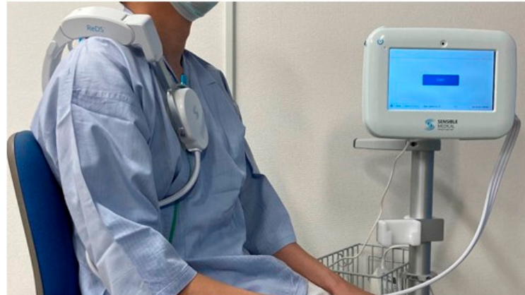
Figure 1. ReDS system. A patient is asked to sit on a chair with a back seat under natural breathing. The patient wears a ReDS sensor and waits for approximately 60 s. The ReDS value, a representative of the percentage of lung fluid amount, is displayed on the screen.
