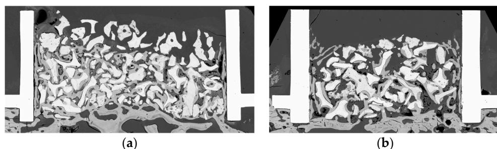
Figure 4. (a) Focused ion beam scanning electron microscopy image of one of the cases treated with 1% metformin. Note the absence of biomaterial in much of the third most distal to the shell of the interior of the cylinder. (b) Focused ion beam scanning electron microscopy image of one of the control cases. Note the absence of biomaterial in much of the third most distal to the shell of the interior of the cylinder.
