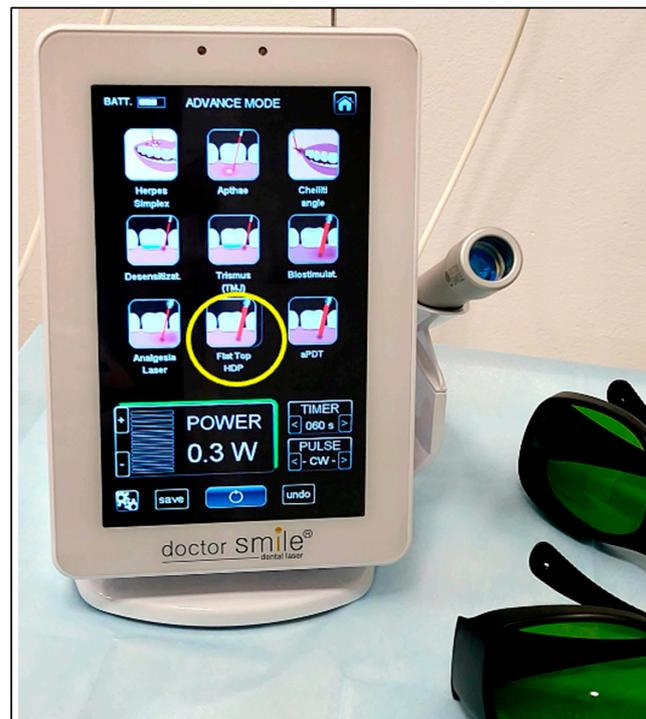
**Figure 1.** The laser device of  $\lambda$  980 nm where the yellow circle indicates PBM therapy with a delivery system of flattop beam profile, and the panel also shows the therapeutic power output “0.3 W”, irradiation time “60 seconds (s)” and emission mode “continuous emission mode (CW)” which were utilised in the study. Eyewear protection (Green in colour) was worn by the operator, patient, nurse and patient’s parent.
