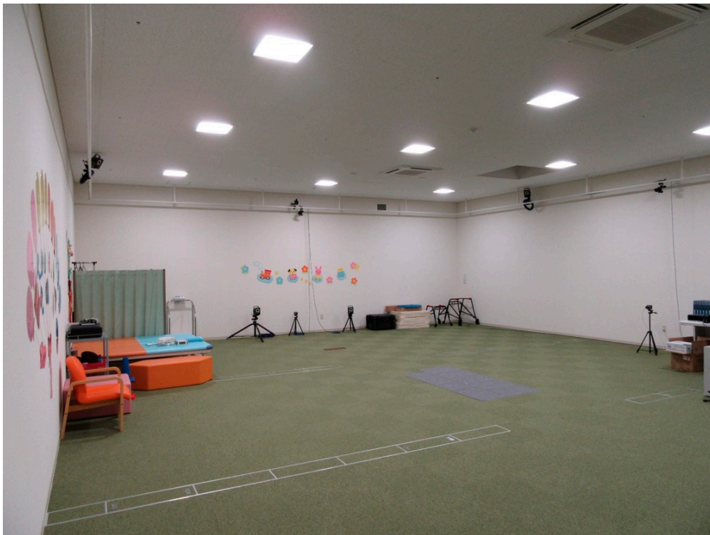
Figure 1. Three-dimensional motion analysis system. The system consists of eight strobe cameras mounted from the ceiling or floor and eight force plates placed in the middle of the walkway.
