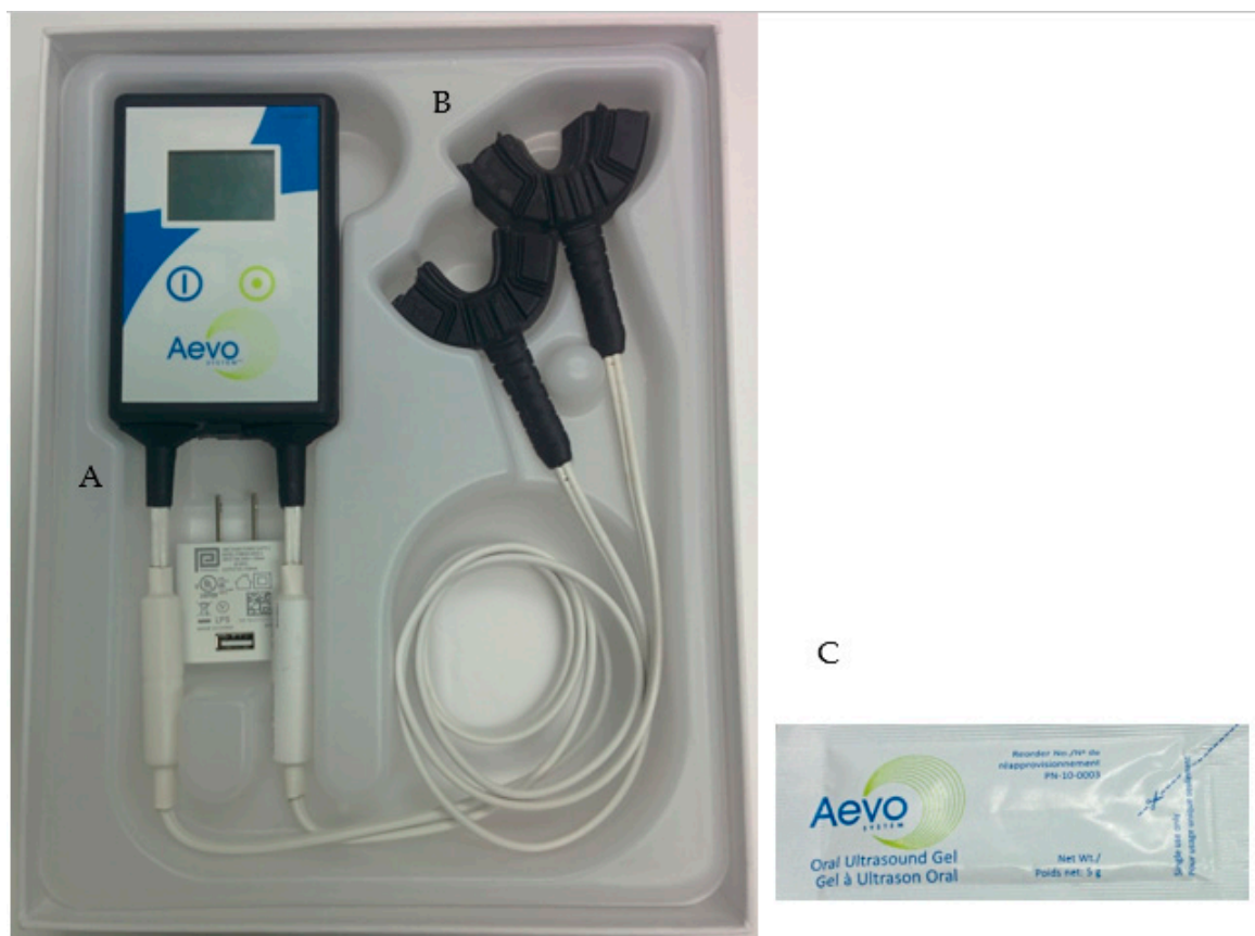
Figure 1. Low-intensity pulsed ultrasound (LIPUS) device (Aevo System). (A): Handheld electronics; (B): mouthpieces; and (C): ultrasound coupling gel.
