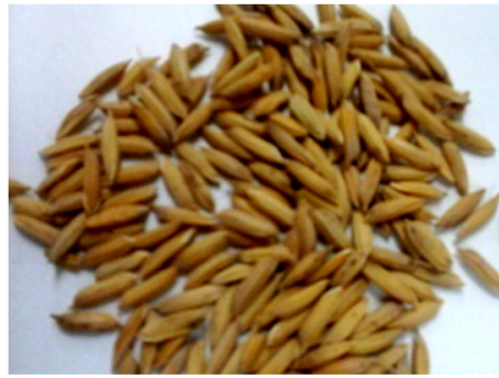
Figure 9. Rice grains after convective drying process at 60 °C ( M_o = 34.5\% dry basis, t = 960 min).
