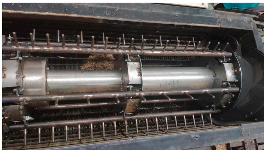
**Figure 5.** Threshing device for individually adjusting threshing rod elongation.
