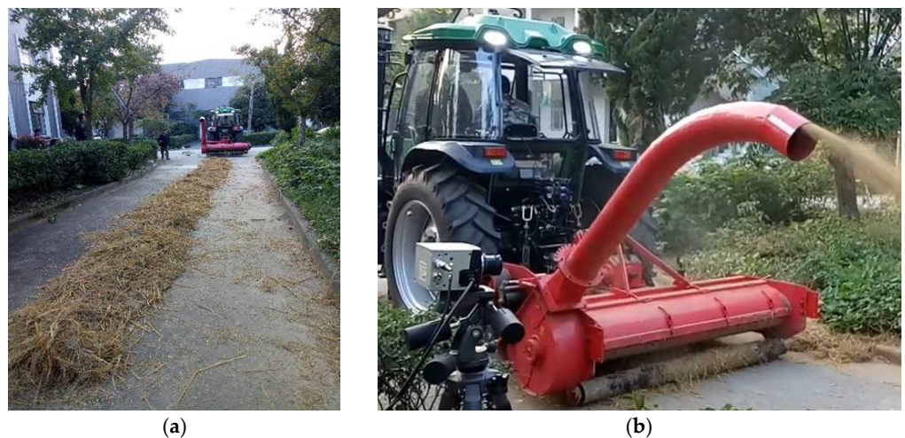
Figure 11. The scenario of verification test: (a) the simulative residual straw; (b) the operation process of back-throwing device.
