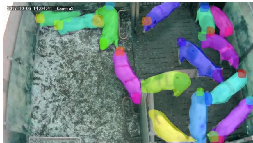
Figure 7. Visualization of the object detection of pigs, their heads and their tails by Mask R-CNN.
