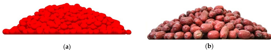
Figure 7. The angle of repose results; (a) simulation test angle of repose, (b) physical test angle of repose.
