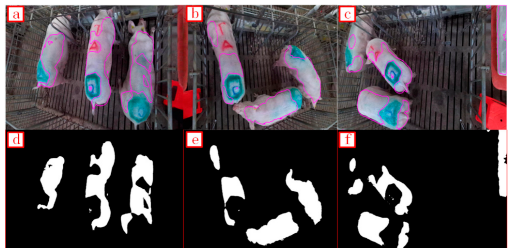
Figure 9. The target detection using UNet-Attention model, (a) without adherence; (b,c) with adherence. The pink outline is the segmentation outcome. The (d–f) are the processing binary diagrams of (a–c), respectively.
