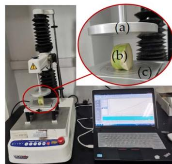
**Figure 12.** Radial compression experiment of broccoli stem: (a) upper indenter; (b) broccoli stem; and (c) fixed platform.
