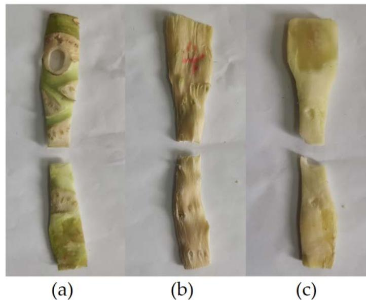
**Figure 23.** The broccoli stem with stretching failure: (a) rind; (b) xylem; and (c) pith.
