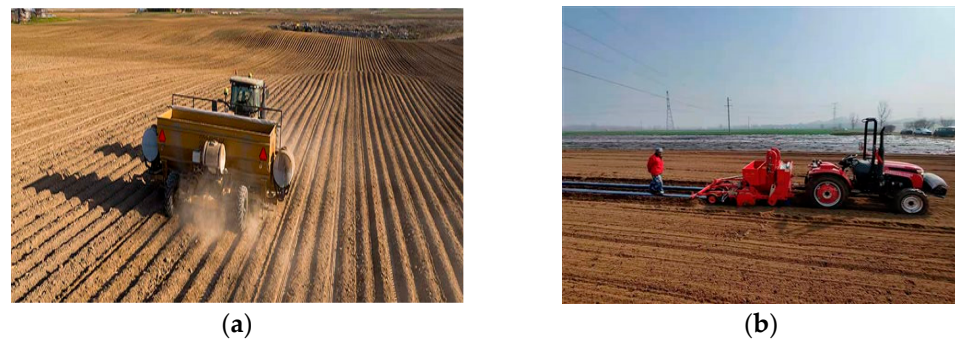
Figure 32. Automatic Potato planter with GPS system. (a) Double L planter works under GPS navigation. Reprinted with permission from ref. [12]. Copyright 2021 Double L Industries. (b) Navigation test of planter.
