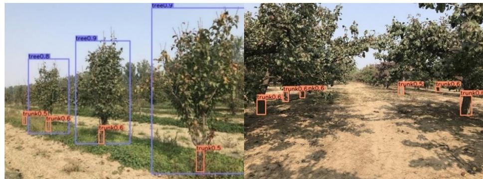
Figure 8. Detection results of tree and trunk under strong sunlight.
