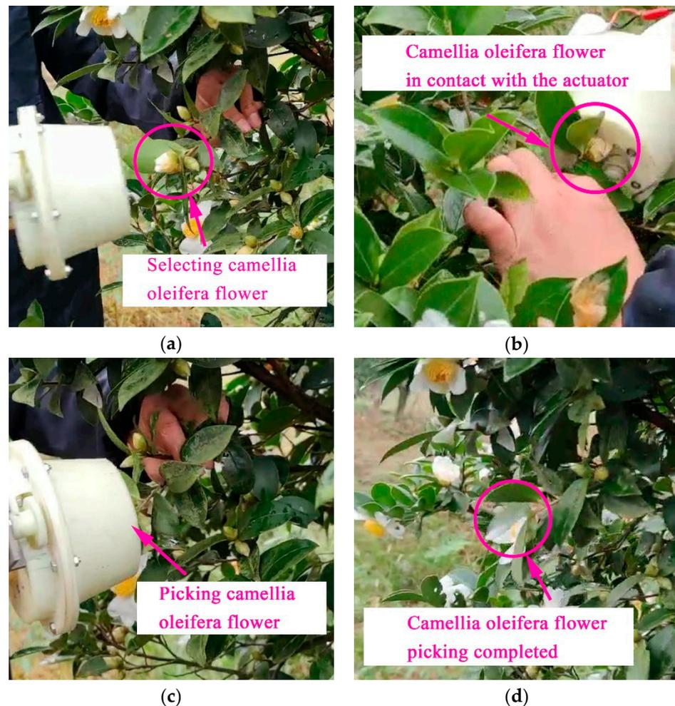
**Figure 14.** Experimental process diagram of the prototype harvesting system for the *Camellia oleifera* flowers. (a) Find flowers. (b) Flower entry actuator. (c) Start picking. (d) Picking is complete.
